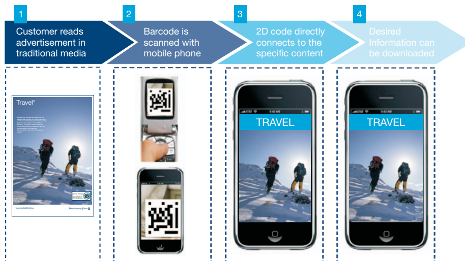
Figure 20: How 2D barcode technology connects print, mobile and online media
